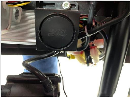
**Security Alarm System** – The alarm system plugs directly into the controller via two connectors. When replacing, separate the original alarm system connectors, dismount, and install the replacement using the same controller connectors. There is a 8mm nut and Philips
