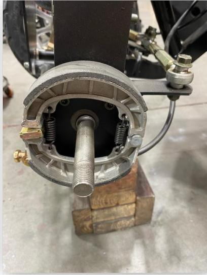
The brake pads are held onto the axle's brake pad catch, and to the actuating brake tension arm with spring tension. Pull the two sides of the brake pads away from each other to remove, and duplicate the reinstall the new pads
