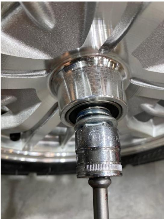
A jack or stand will be needed to remove the front tire. The front wheel is secured by the front axle bolt. On the wheel nuts there will be covers that need to just be popped off. The size you're going to need is going to be a 19mm socket to take this off.
