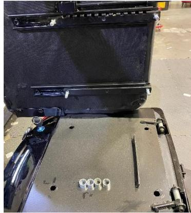
Remove all 4 bolts using a **13mm** socket with a ratchet. Be careful as there are 4 spacers as well that will be.
