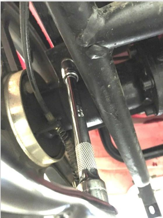
There are two transaxles to swing arm bolts on each side of the scooter. The bolt size is going to be . Make sure the bolts are tight on each side. If there is a gap between the axle bracket and the swing arm, this is normal. If overtightened bolts from the transaxle to swing arms can potentially snap.
