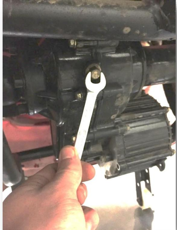
It is recommended to change the transaxle oil between from one to three years. Unlike a gasoline engine, the motor does not require a specific amount of oil to operate properly. It is strictly the lubrication method to avoid overheating in the differential assembly. There is a drain and fill bolt on the top and bottom of the motor. Drain old oil, replace fill bolt, and use 10W-30 motor oil to refill the transaxle, with approximately  $\frac{1}{2}$  quart.
