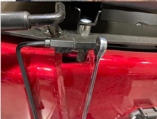
The seat is securing by two bolts, and the seat latch. The seat bolts are a 5mm hex head bolt on the bolt side, and 10mm on
