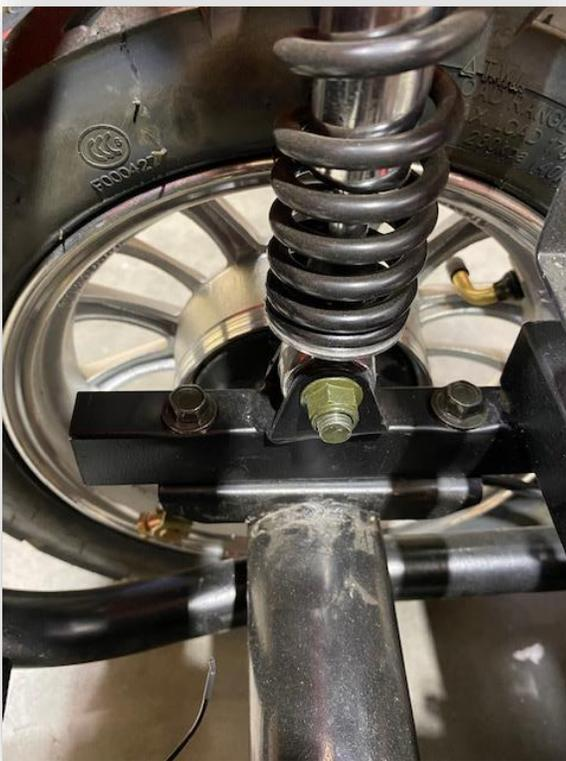
Once the rear wheels are removed, the next step is to remove the four 14mm axle to swing arm bolts. These bolts secure the transaxle assembly to the swing arms.
