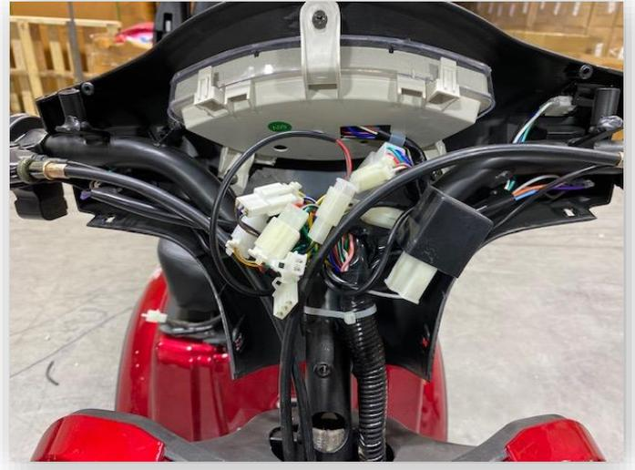
**Throttle Replacement** – To replace the throttle, start by removing the headset shroud. Once removed, separate the original throttle's electrical connector, and loosen (but do not remove) the 3 MM set screw for the original throttle. Disconnect both connectors and your job is complete.
