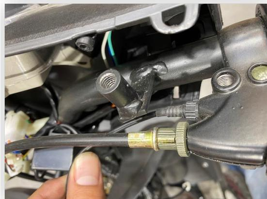
adjuster with securing washer to the point where the adjuster and washers cut outs match up with the cut out for the brake handle.
