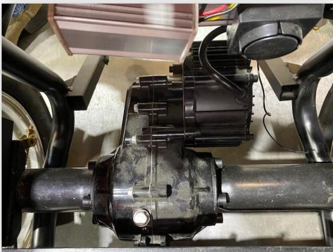
Going internal with the motor to determine if the differential, transfer case, motor hall sensors, or other internal components is the issue is not recommended for field service technicians. Typically, the labor costs for disassembling, testing, and reassembling will exceed the cost for a replacement motor. If the control unit is emitting the proper power to the motor under load, the brake sensor is not activated, and the rheostat is unplugged, and the motor is not engaging,
