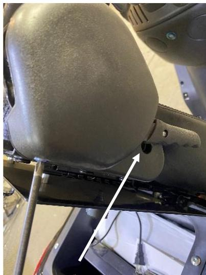
*(The back rest will the come off once all bolts are removed on each side in above photo )*
