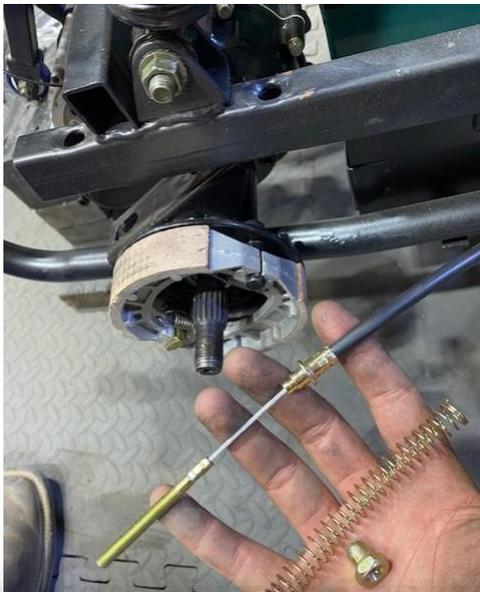
You will be using a 10 mm allen wrench and a 19 mm socket wrench to loosen the nut to take the axle bolt off.
