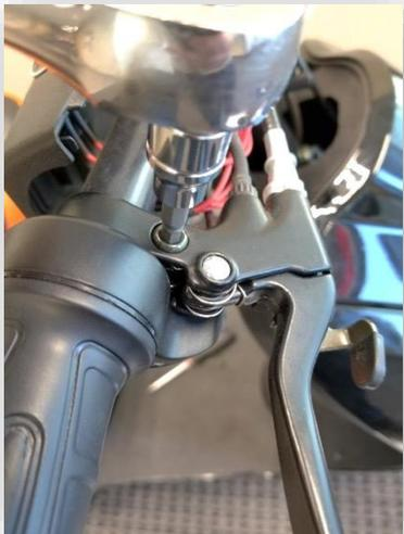
**Right (Front) Brake Handle Replacement** – To replace the right brake handle, start by removing the headlight shroud. Once removed, separate the brake handle’s electrical connector. Once separated, remove any tension from the brake line by taking off the adjustment nut on the opposite end of the brake cable. Then, remove the cable from the brake handle as demonstrated in the photos below.
