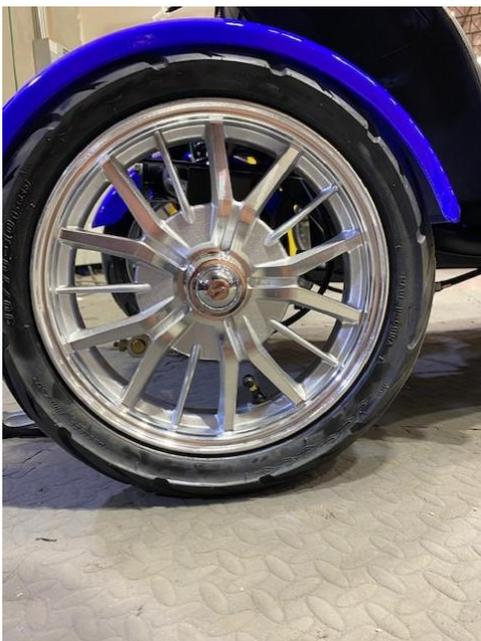
A jack or stand will be needed to remove the front tire. The front wheel is secured by the front axle bolt. On the wheel nuts there will be covers that need to just be popped off. The size your going to need is going to be a 19mm socket to take this off.
