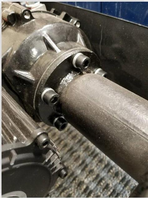
The final step is to remove either side axle assembly. When either axle is removed, the remaining axle that is still connected to the motor will have room to be able to drop away from the frame. Both axles are secured by five 6mm hex (Allen wrench) bolts. Ensure the motor to axle seal is salvaged is just the axle or motor is being replaced.
