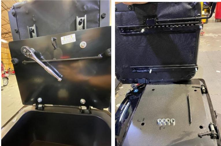
**Step Three** – Remove all 4 bolts using a **13mm** socket with a ratchet. Be careful as there are 4 spacers as well that will be
