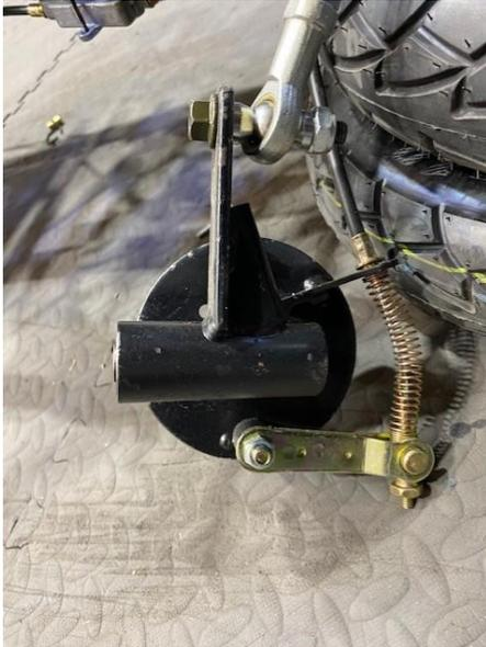
Once the brake cable hardware is removed, the brake line will have no tension. Remove the cable from the brake handle next by turning the barrel adjuster with securing washer to the point where the adjuster and washers cut outs match up with the cut out for the brake handle.
