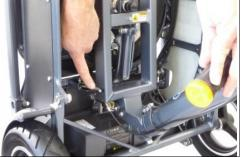
While pushing the handlebar down and inwards release the 'E' latch.
