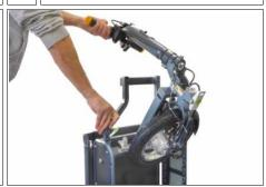
Pull the steering column up and over the carry handle until it **locks** in place.
