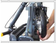
7 Release the front wheel by a sharp pull or twisting.
