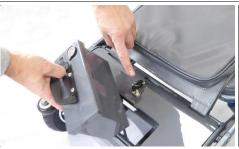
Remove the battery by unlocking using the key and applying gentle pressure.
