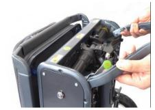
Press the steering column in to the frame until latch 'E' locks.
